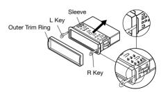
5. Mount the sleeve by inserting the sleeve into the opening of the dashboard and bend open the tabs located around the sleeve with a screwdriver. Not all tabs will be able to make contact, so examine which ones will be most effective. Bending open the appropriate tabs behind the dashboard to secure the sleeve in place.
